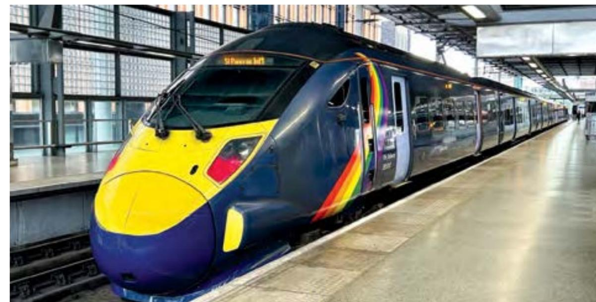
UK Rails' first refurbished Class 395 Javelin re-entered passenger service in August 2023 with new seats and carpets, USB at-seat power sockets and LED lighting.
