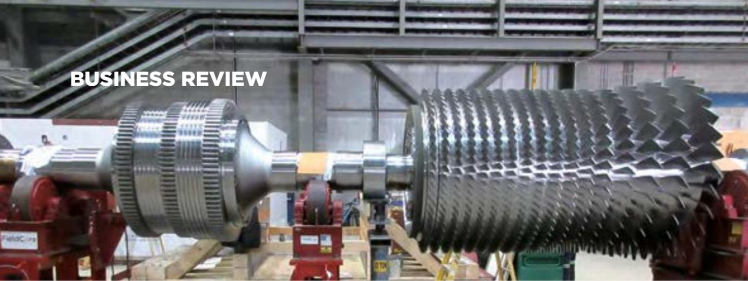
Canadian Power's Meridian cogeneration plant carried out the replacement of a rotor for one of its two gas turbines.
