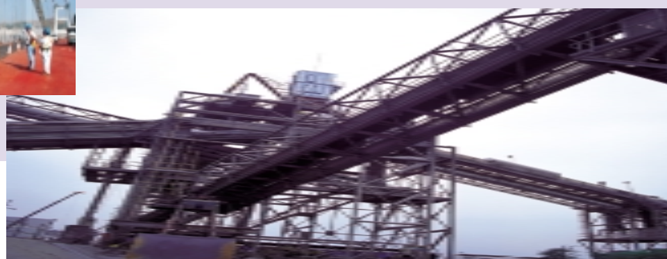
Belt conveyors are extensively used in the Tap Shek Kok cement plant for bulk material transportation.
